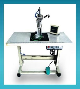
Description: This machine mainly USES the principle of ultrasonic wave, used for welding the earband of plane, cup and other opposite sex masks. Stable output, reliable performance, easy to operate, beautiful solder joints, no damage to the material.
